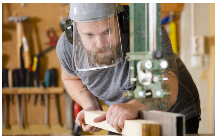
The bandsaw is a powered tool used to cut curved lines through thin material.
