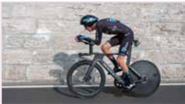
Bike technology in road cycling has undergone significant advancements in recent years. Bike frames are made of **carbon fibre** which is a very light but strong material and contributes significantly to improving aerodynamics. The sleek, streamlined frames reduce air resistance, allowing the bike (and rider) to cut through the air more efficiently.
