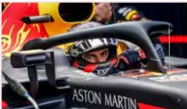
The **halo** is a significant addition to the safety features of Formula 1 cars. The halo is a curved bar made of titanium that is positioned above the driver's head and in front of the cockpit. It contributes to head protection, debris deflection and forms an enhanced roll bar.
